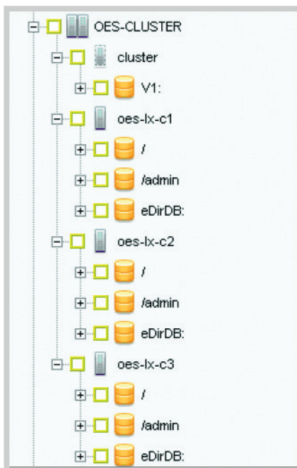
Illustration 1. In this DPX screen capture, the virtual node is labeled as "cluster." The item "V1" represents the shared resource. Objects oes-lx-c1, oes-lx-c2, and oes-lx-c3 are the server nodes in the cluster.
