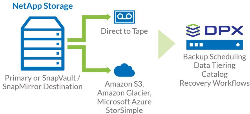
*DPX provides easy backup of NetApp file data to either tape or cloud. The DPX server manages the backup scheduling and data tiering and maintains a catalog of files. Recovery workflows are also managed by DPX, whether restoring from tape or from cloud.*
