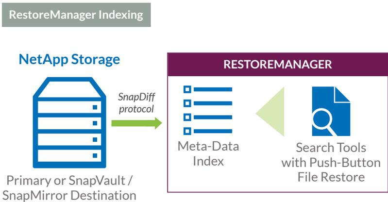
*RestoreManager uses the SnapDiff protocol to create a meta-data index of all copies on NetApp primary and secondary storage. The index can be easily searched, and one or more files recovered with a single click.*
