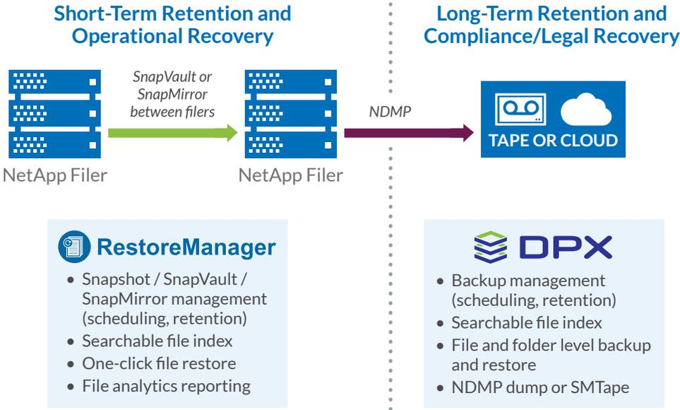
*This diagram provides a high-level look at the Catalogic solution. RestoreManager software provides file search and restore for daily operational recovery, while DPX provides long term retention of data on tape or cloud. SnapVault and SnapMirror are optional and NDMP backups can be taken directly from the primary NetApp filer.*
