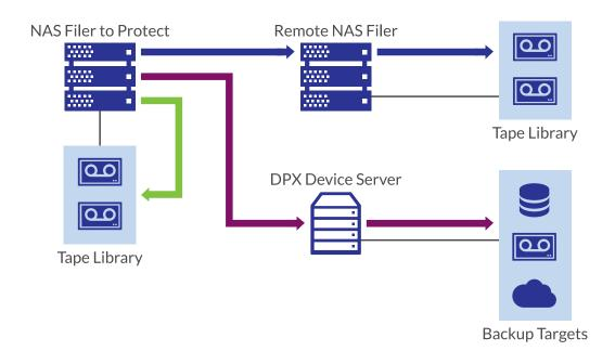
LOCAL NDMP BACKUP Filer to directly attached tape library **FILER-TO-FILER NDMP BACKUP** Filer to filer to tape library
